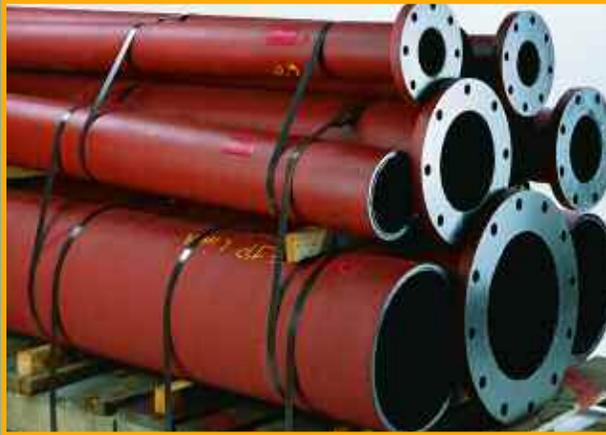
Pipe is fabricated with different end configurations and in sizes 3" to 42" and in lengths up to 20 feet. Fabricated pipe is bundled and packaged for shipment to the jobsite.
